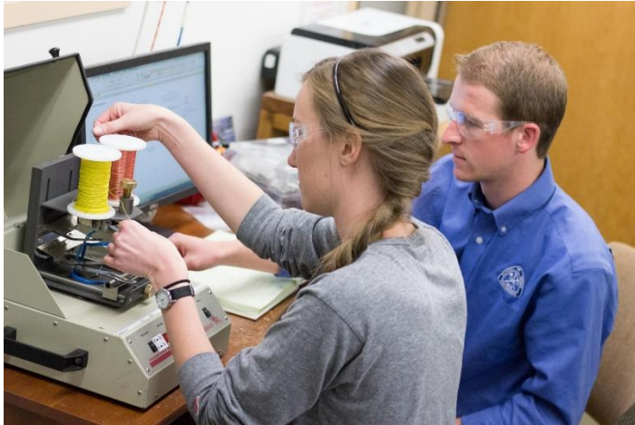
Ginny Judge and Blake Whitley spot welding thermocouple to sample
