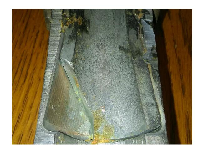
Carbide broke due to cobble at 205,000 tons but the carbide was still in good enough condition to have been used further.
