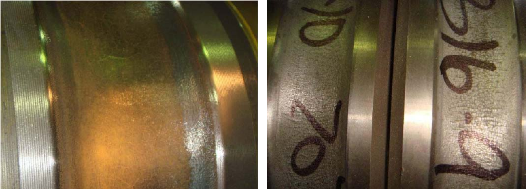
Figure 1: Roughing Mill and Finishing Mill Rolls experiencing fire cracks.
